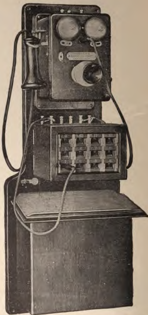
FIG. 200.—Combined station apparatus and switchboard for use in small exchange hotel systems. The drop-jack here used is the one described on pages 156-158
